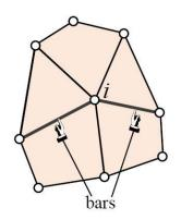
A finite element *patch trial function* is the union of shape functions activated by setting a degree of freedom at that node to unity, while all other freedoms are zero. A patch trial function "propagates" only over the patch, and is zero beyond it.
