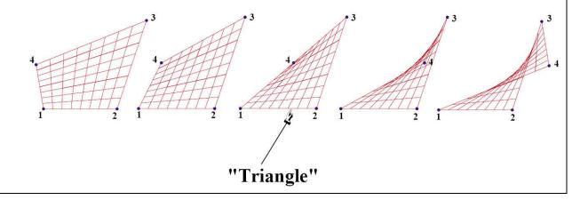
For higher order elements proper location of corner nodes is not enough. The non-corner nodes (midside, interior, etc.) must be placed sufficiently close to their natural locations (midpoints, centroids, etc.) to avoid violent local distortions. The effect of midpoint motions in quadratic elements is illustrated in Figures 19.3 and 19.4.
