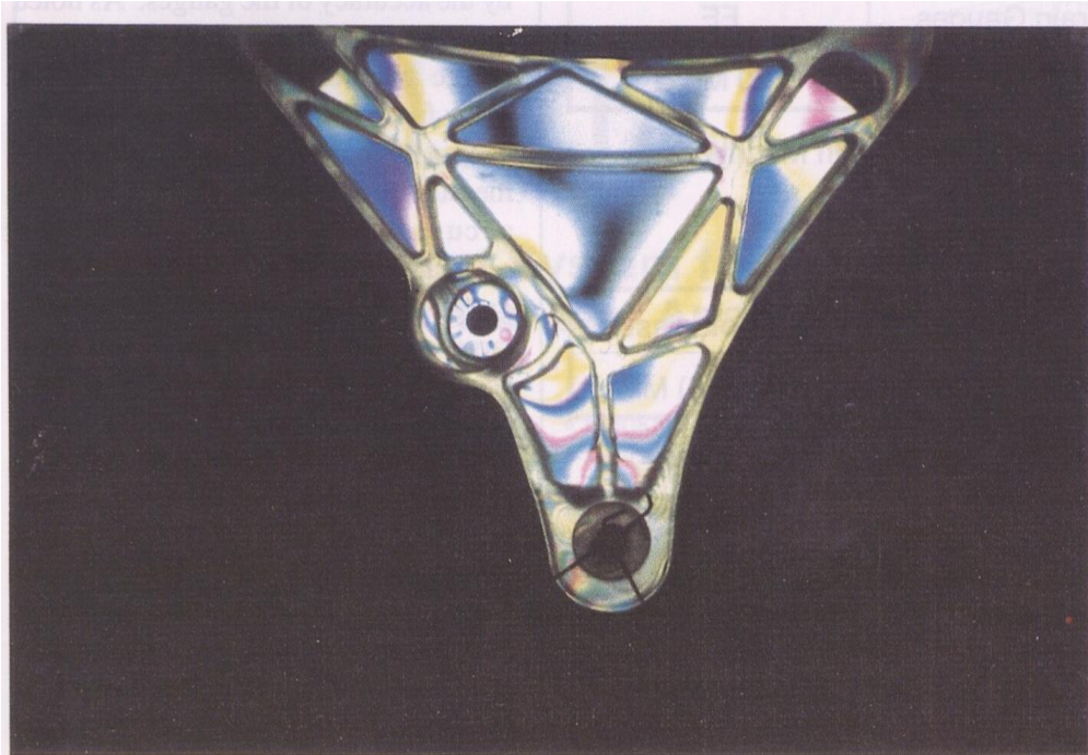
Figure 2. Photoelastic Plot of Overall Stress Distribution
