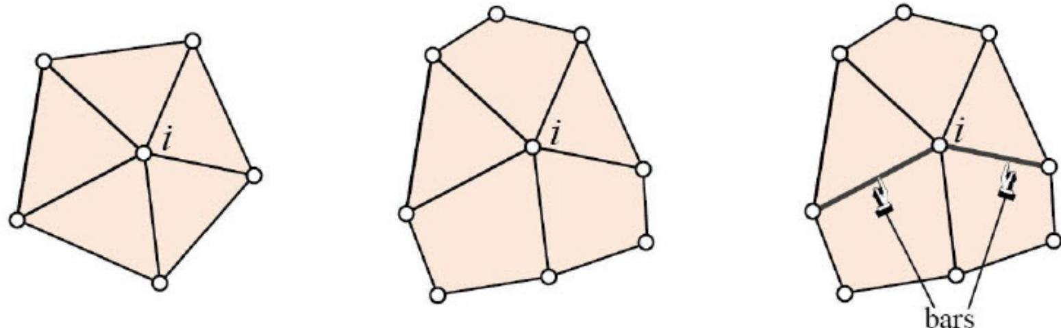
A finite element *patch trial function* is the union of shape functions activated by setting a degree of freedom at that node to unity, while all other freedoms are zero. A patch trial function "propagates" only over the patch, and is zero beyond it.
