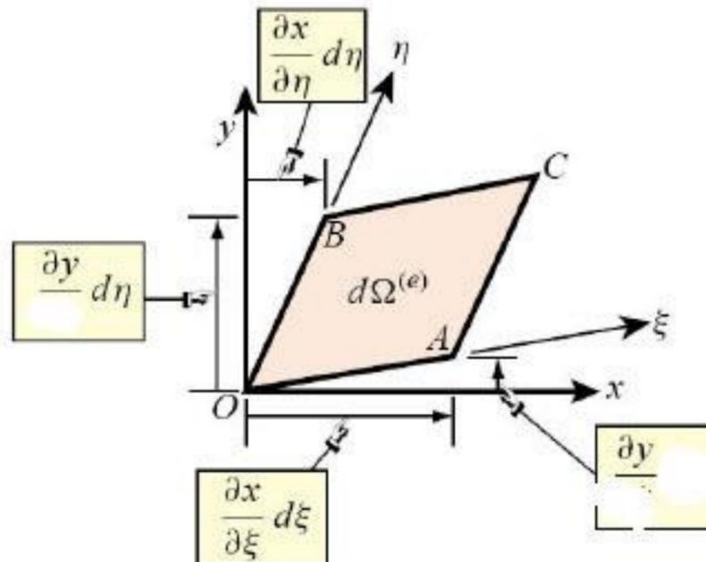
$$dA = \vec{O}B \times \vec{O}A = \frac{\partial x}{\partial \xi} d\xi \frac{\partial y}{\partial \eta} d\eta - \frac{\partial x}{\partial \eta} d\eta \frac{\partial y}{\partial \xi} d\xi = \begin{vmatrix} \frac{\partial x}{\partial \xi} & \frac{\partial y}{\partial \xi} \\ \frac{\partial x}{\partial \eta} & \frac{\partial y}{\partial \eta} \end{vmatrix} d\xi d\eta = |\mathbf{J}| d\xi d\eta.$$
